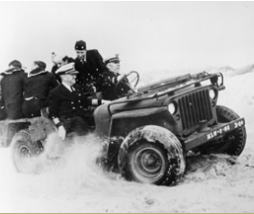
Navy brass testing out high flotation tires on an unidentified prototype Jeep. Note the capstan winch on the front.
